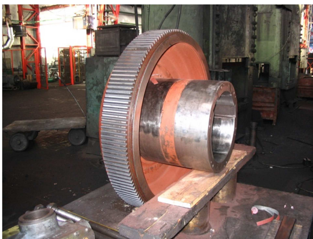
Fig. 4. Appearance serrated coupling hub.
